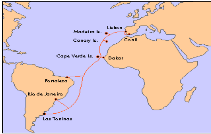
Figure: 2.15: Atlantis 2 Cable - Source: The existing fiber connectivity in Africa, Pre-study Report, Royal Institute of Technology, Stockholm, October 2003
