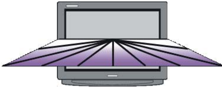
Measuring from the directions of 0^\circ, \pm 30^\circ, \pm 45^\circ, \pm 60^\circ, \pm 75^\circ or from the continuous direction of -90^\circ to +90^\circ on the horizontal plane
