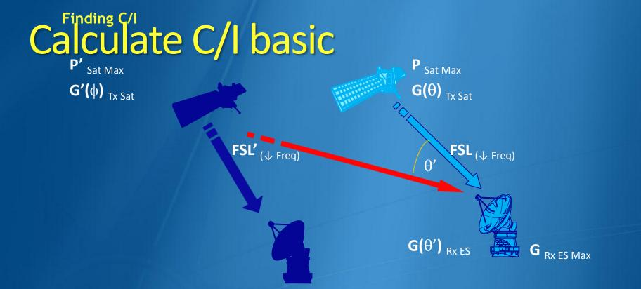
$C \downarrow = P_{Sat Max} + G(\theta)_{Tx Sat} + G_{Rx ES Max} - FSL_{(\downarrow Freq)} (dBW)$  $I \downarrow = P'_{Sat Max} + G'(\phi)_{Tx Sat} + G(\theta')_{Rx ES} - FSL'_{(\downarrow Freq)} (dBW)$  $C/I \downarrow = C \downarrow - I \downarrow (dB)$
