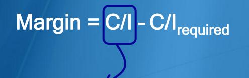
C/I: Carrier to Interference (dB)
