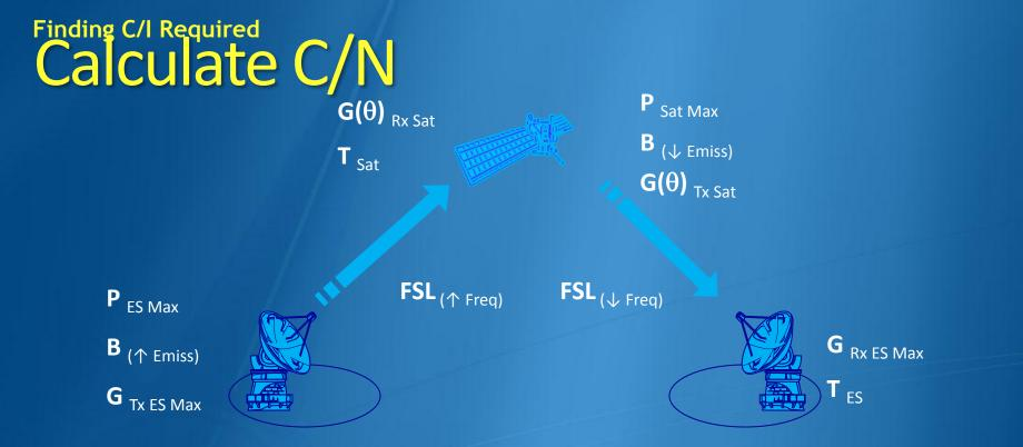
Uplink C/N  $C/N \uparrow = P_{ES Max} + G_{Tx ES Max} + G(\theta)_{Rx Sat} - FSL_{(\uparrow Freq)} - (k + T_{Sat} + B_{(\uparrow Emiss)}) (dB)$ Downlink C/N  $C/N \downarrow = P_{Sat Max} + G(\theta)_{Tx Sat} + G_{Rx ES Max} - FSL_{(\downarrow Freq)} - (k + T_{ES} + B_{(\downarrow Emiss)}) (dB)$
