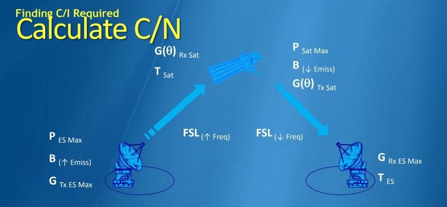
Maximum Peak Power Necessary Bandwidth of Emission Maximum Earth Station Antenna Gain Free Space Loss (assigned frequency) Off-axis Satellite Antenna Gain Receiver System Noise Temperature Service Area
