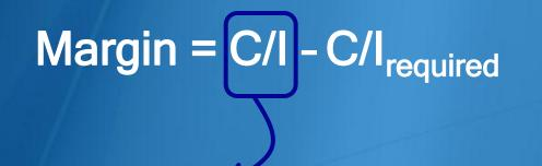
C/I: Carrier to Interference (dB)
