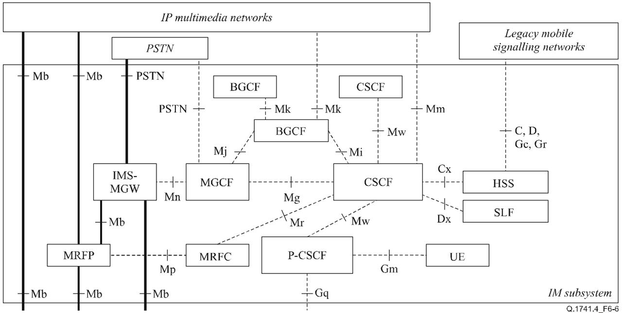
**Figure 6-6/Q.1741.4 – Configuration of IM Subsystem entities**
