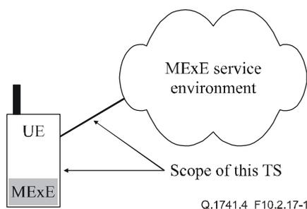
**Figure 10.2.17-1/Q.1741.4 – Scope of Technical Specification 22.057**
