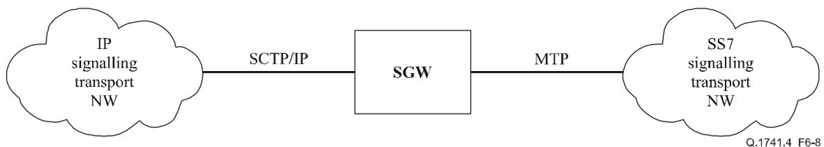
**Figure 6-8/Q.1741.4 – Configuration of a Signalling Gateway function**
