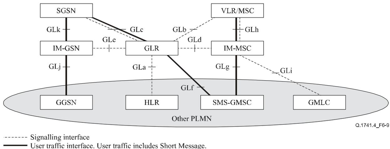
**Figure 6-9/Q.1741.4 – Configuration of a PLMN and interfaces with GLR**
