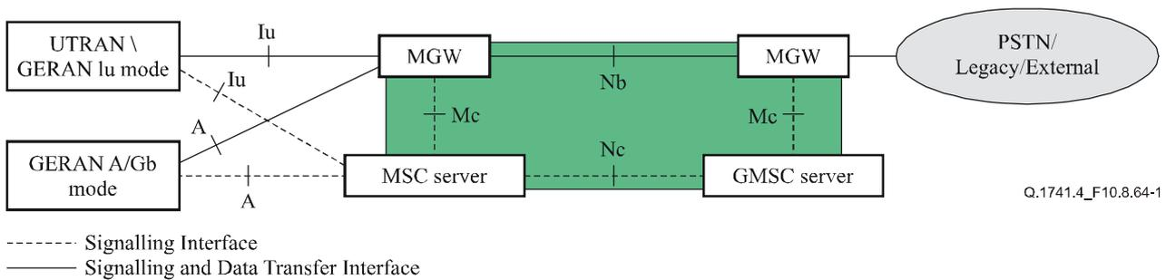
**Figure 10.8.64-1/Q.1741.4 – CS core network logical architecture**
