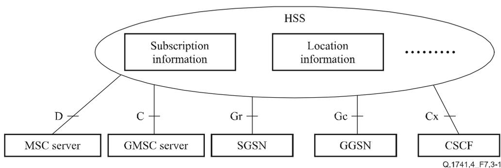
**Figure 7.3-1/Q.1741.4 – Example of a generic HSS structure and basic interfaces**
