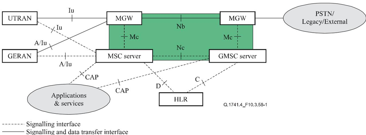
**Figure 10.3.58-1/Q.1741.4 – CS core network logical architecture**
