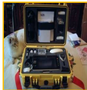
(b) «Nomad solutions» – Waterproof and secure equipment – ECG, SpO 2 , Spirometer, Glucometer, Rapid tests; autonomy : 3 hours, transmission: GSM/GPRS/3G satellite; weight: 3,9 Kg Petitet (2008)
