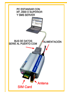
(d) Argentina – secure, mobile phone service for message exchange, the SIM card is located inside the Micro-SIM Type card holder of the modem, Escobar (2009)
