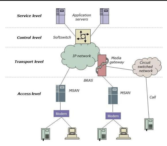
The basic network structure for an NGN core model based on a simple 'all IP' approach, potentially augmented with some traditional TDM networks.
