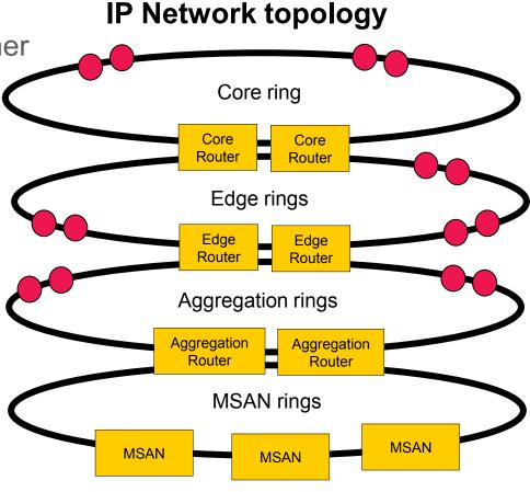
The models typically assume ring structures for redundancy and efficiency although star structures have also been used.
