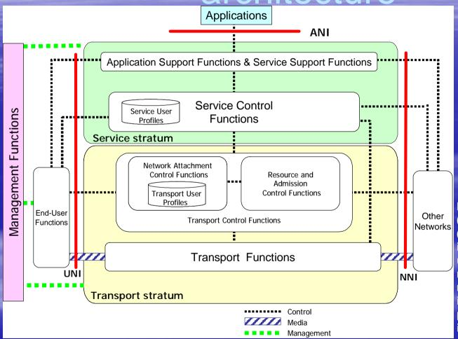
NOTE: The user network interface (UNI), network network interface (NNI), and application network interface (ANI) should be understood as general NGN reference points that can be mapped to specific physical interfaces depending on the particular physical implementations.
