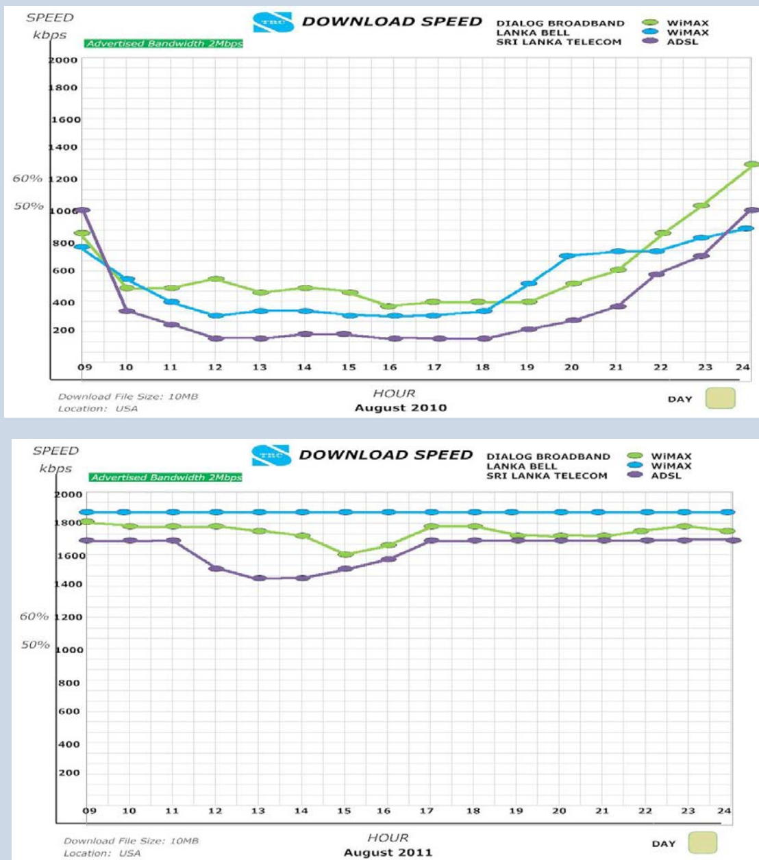
Figure 7: QoS Measurements carried out by TRCSL
