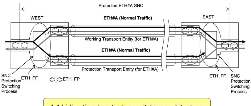
1:1 bidirectional protection switching architecture
