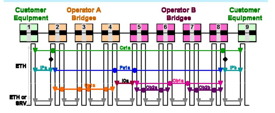
Multiple MEG levels are defined to allow running OAM in different spans
