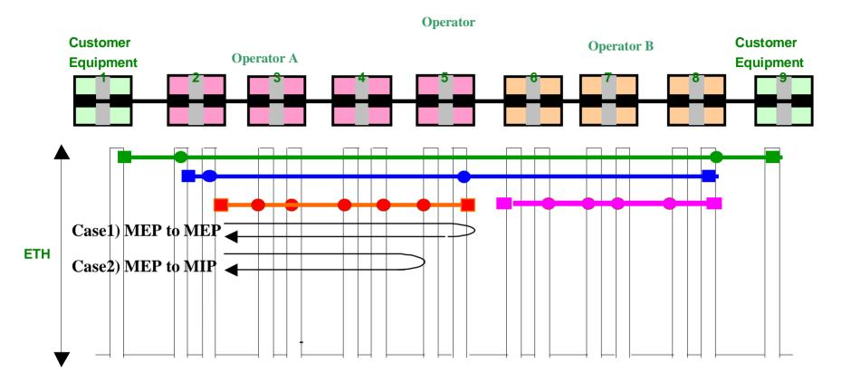
LB is mainly used for connectivity verification changing the test span.
