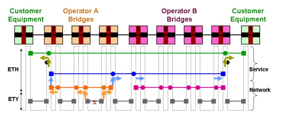
AIS is used for alarm suppression by notifying the bridges in downstream of the existence of the defect and of the fact that it has already been reported (and as such, bridges in downstream need to take no action).
