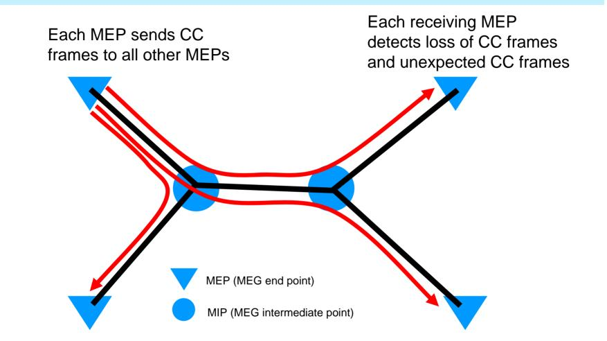
CC can be used for defect detection in multipoint-to-multipoint networks.
