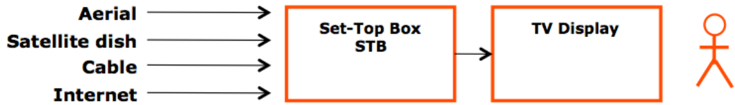
Figure 16: Digital television reception – Set-top box with an existing TV set
