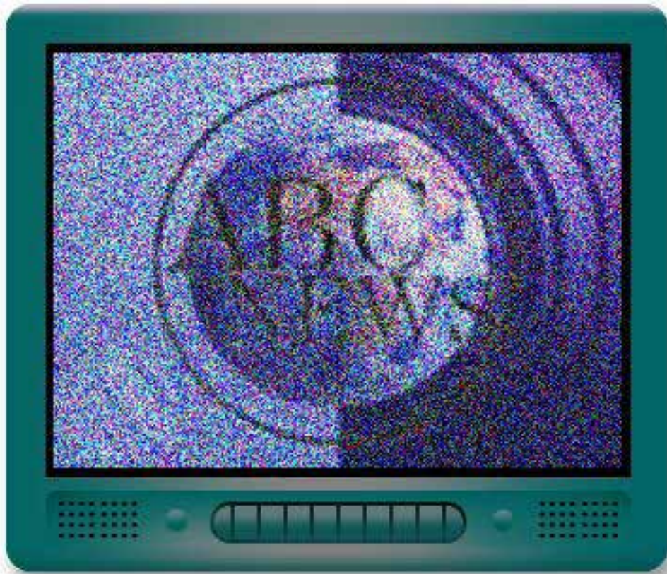
Figure 9: “Snow” on an analogue television picture
