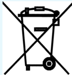
Figure 1: Symbol for use by manufacturers to inform consumers that their ICT equipment is not to be classified as ordinary waste
