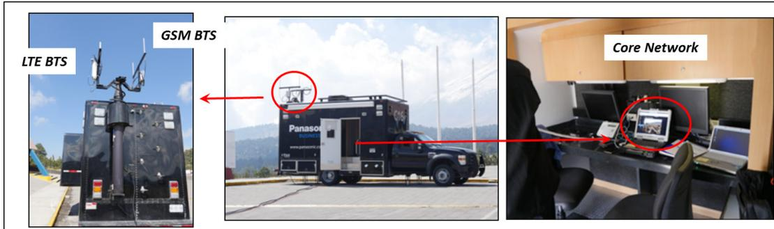
**Figure 11A** shows an example of a local cellular system for GSM and LTE services. This system provides GSM and LTE services via one PC-installed core network function.
