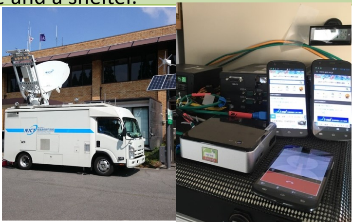
MDRU with NICT's mobile satellite earth station
