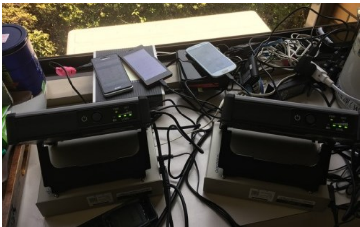
MDRU with satellite-based mobile phones
