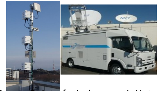
▲ Access Point of wireless mesh Network (left); Mobile Earth Station (right)
