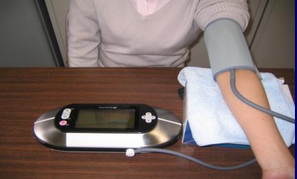
The peripheral device is equipped with memory, an electronic sphygmomanometer, electrocardiograph, electronic signboard, and buttons for answering questions.
