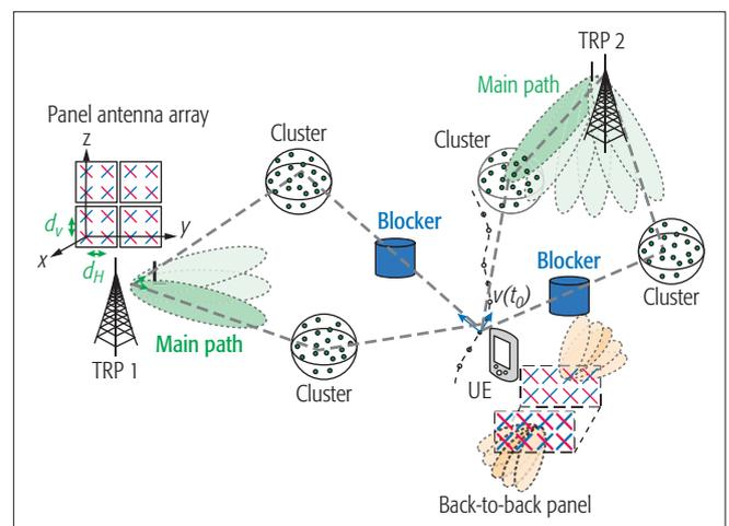
FIGURE 2. Illustration of 5G channel model and system-level simulation scenario.
