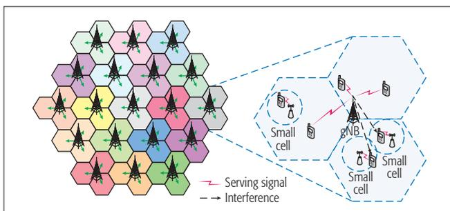
FIGURE 1. A typical network layout of system-level simulation.
