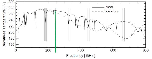
111 The set of frequencies for the measurementof ice clouds centers around 183 GHz, 243 GHz,325 GHz, 448 GHz and 664 GHz 111
