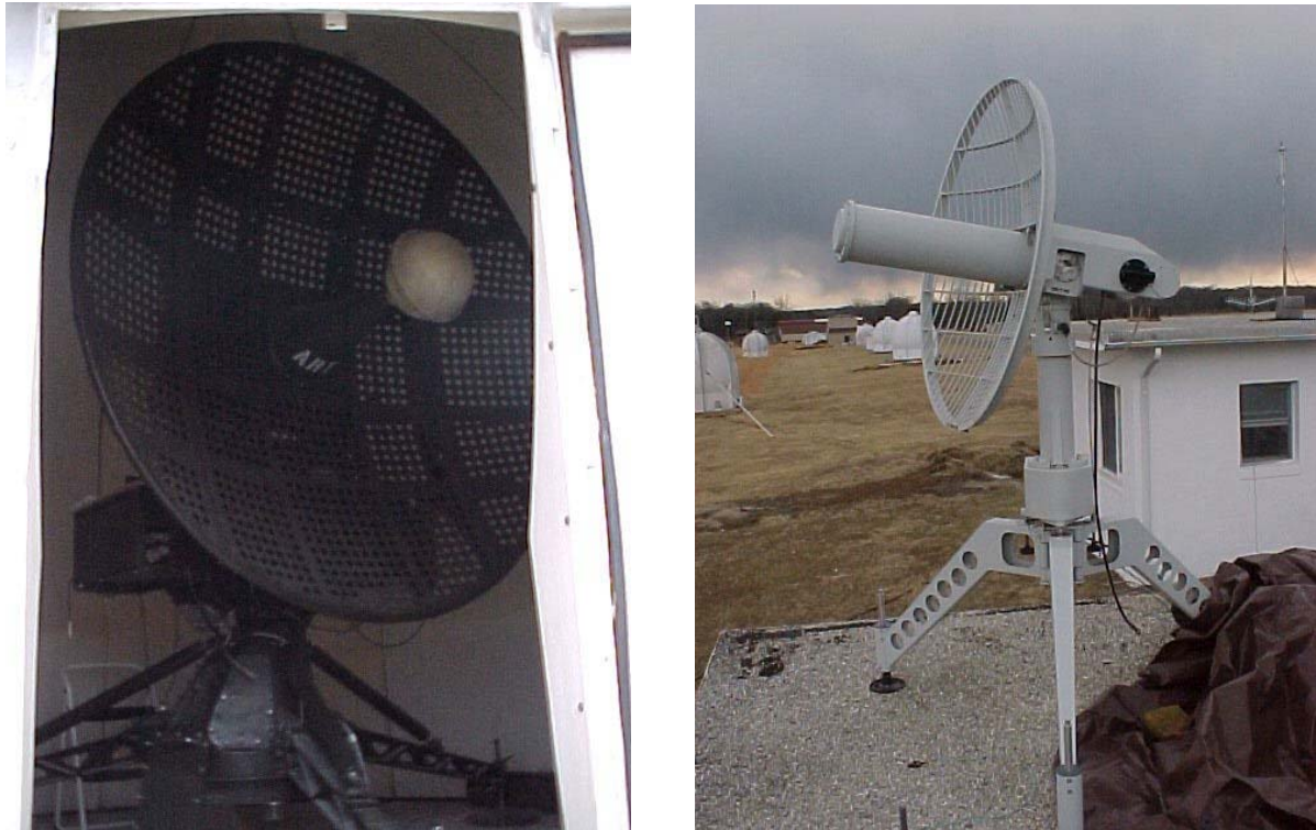
FIGURE 3-7 Tracking antenna systems (1 668.4-1 700 MHz)
