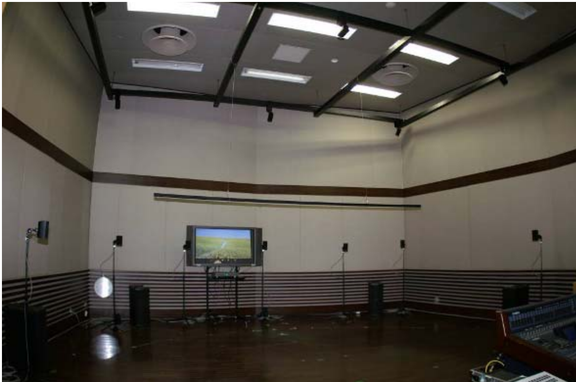
Home 22.2 multichannel sound system using multiple compact loudspeakers
