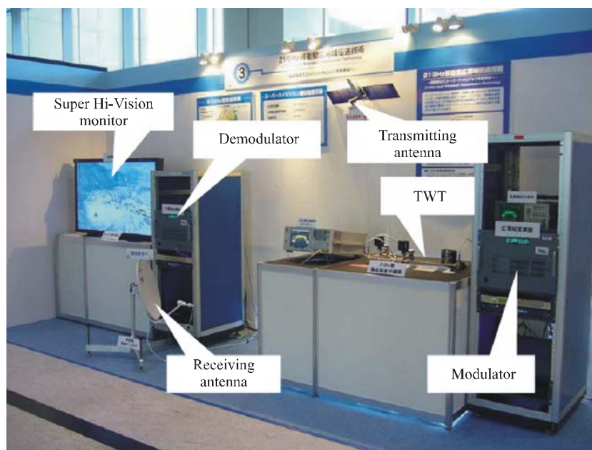
FIGURE 1 Transmission experiment in the 21 GHz-band
