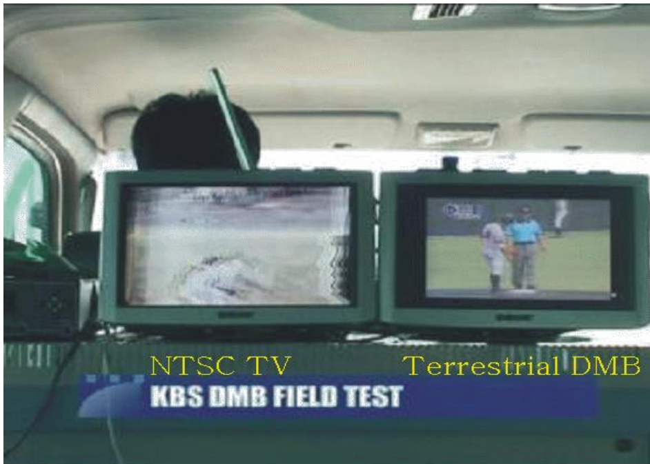
FIGURE 22 Reception comparison between NTSC and T-DMB
