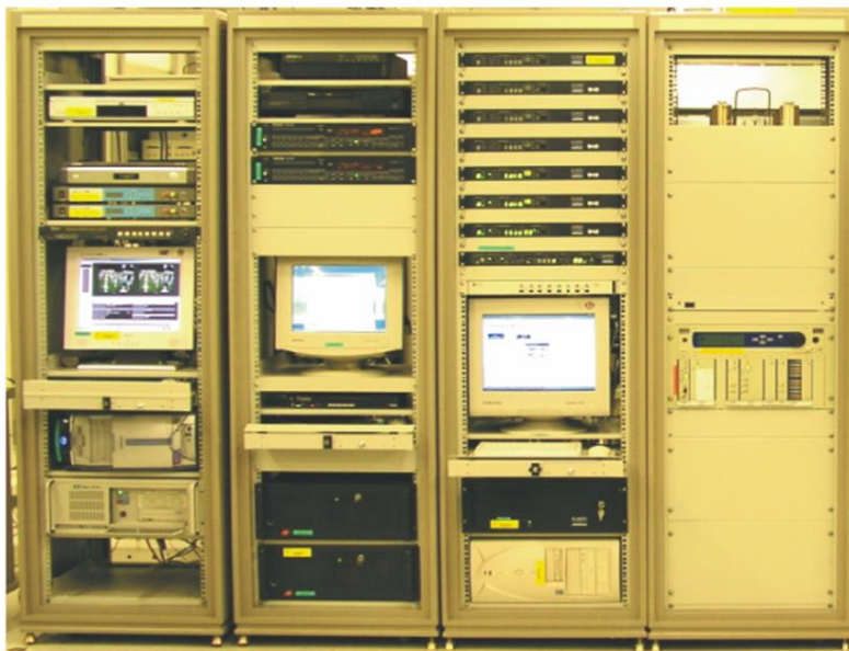
FIGURE 23 A T-DMB transmission system developed for test trial
