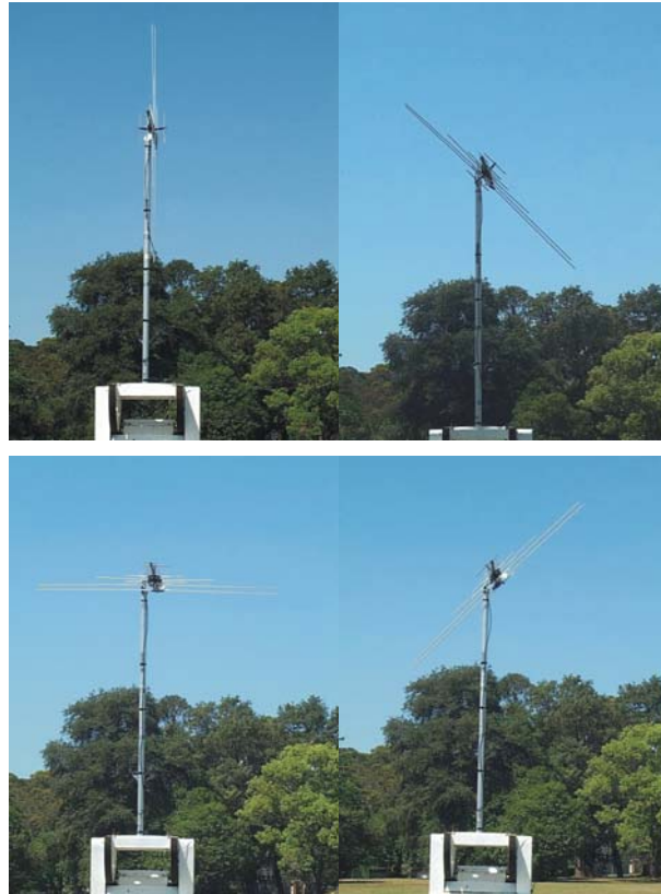
FIGURE 4 Polarization viewed from front of AUT
