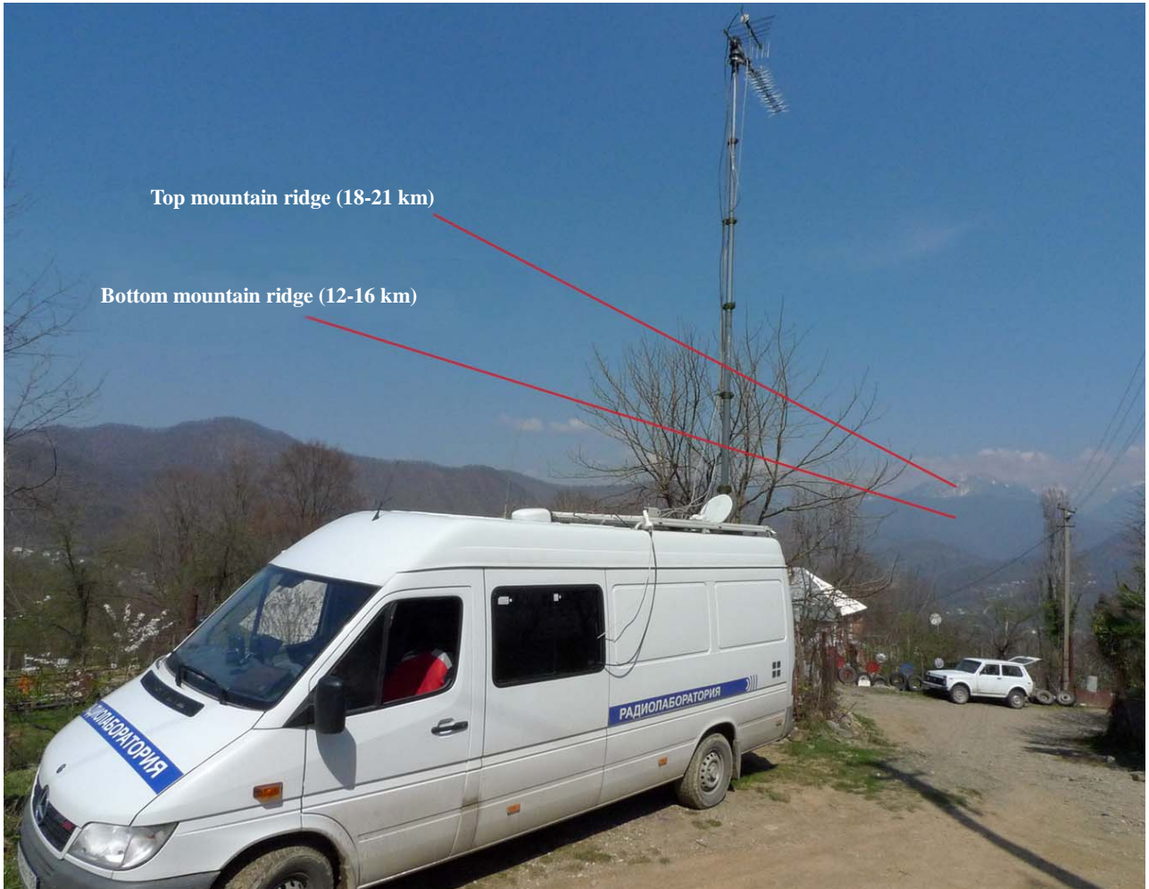
FIGURE 16 Measurements of reflected signal
