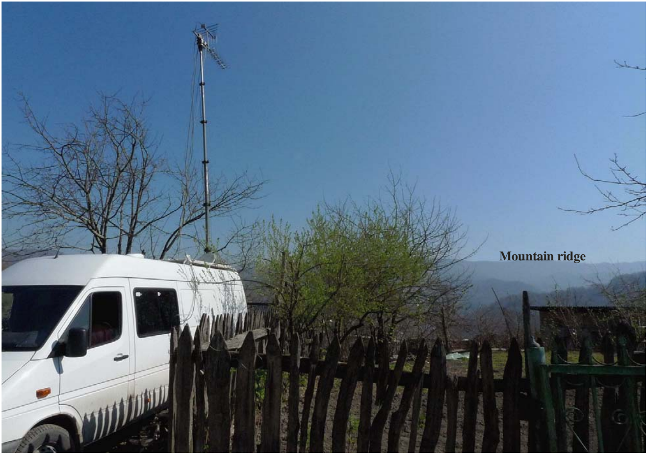
FIGURE 20 Reception of reflected signals at the boundary of coverage area
