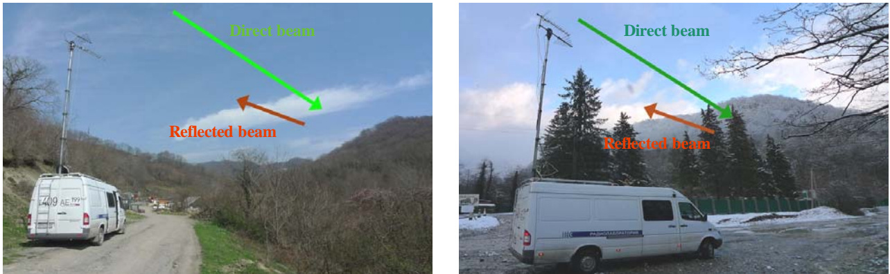
FIGURE 24 Conditions of reflected signal reception in river-valleys
