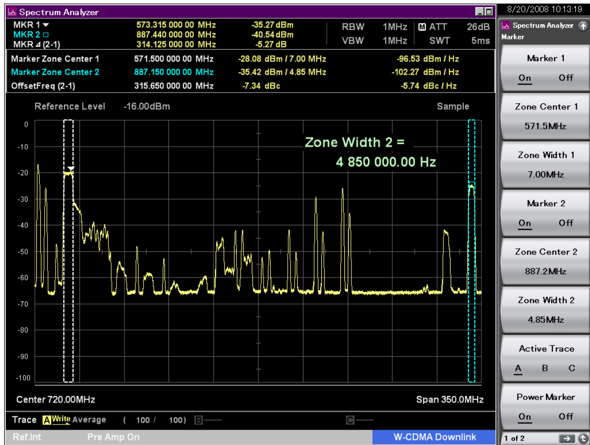
Spectrum chart at St Clair (picked up via external rooftop antenna)
