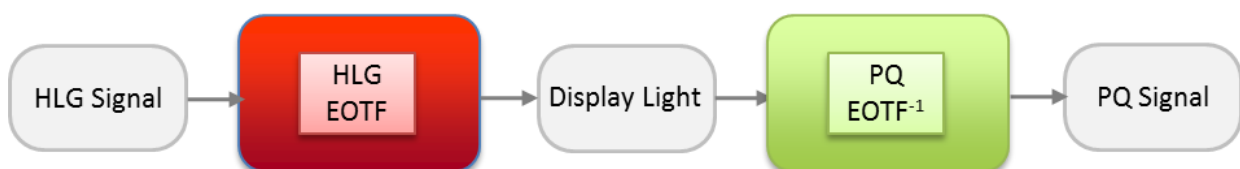
Concept of transcoding from HLG to PQ
