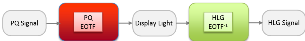
Concept of transcoding from PQ to HLG
