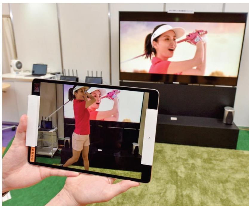
FIGURE 18 Prototype AR content synchronized with TV programme
