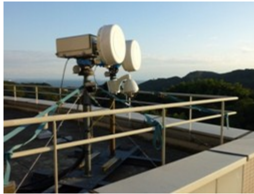
FIGURE 18 Photograph of the transmission experiments using parallel wireless links
