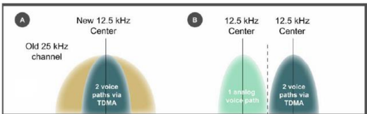
FIGURE 8 Effect of using TDMA technology in an existing 12.5 kHz and 25 kHz channel
