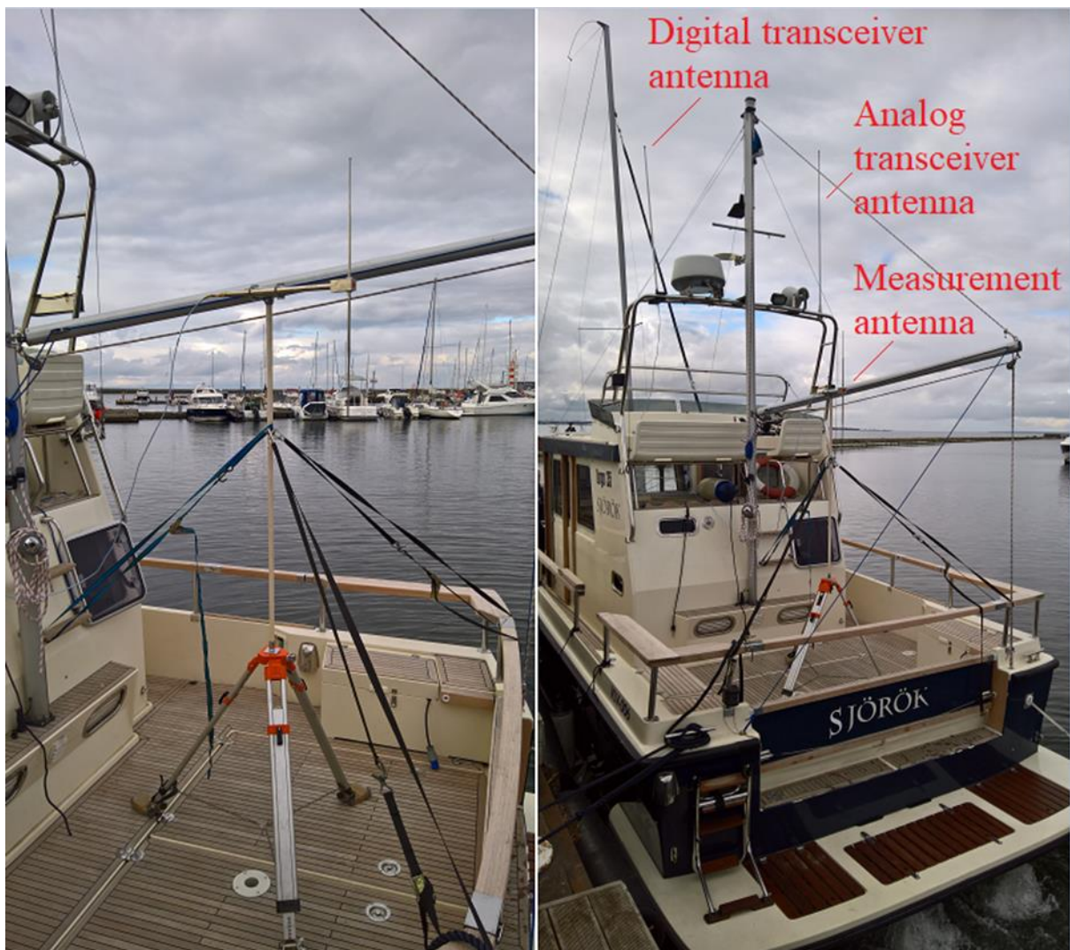
FIGURE 11 Antennas installed on a vessel
