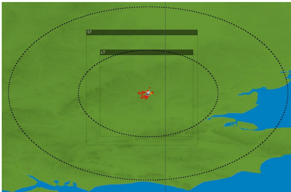
Protection zone for Brookmans Park earth station with respect to Small Cell Indoor (3)
