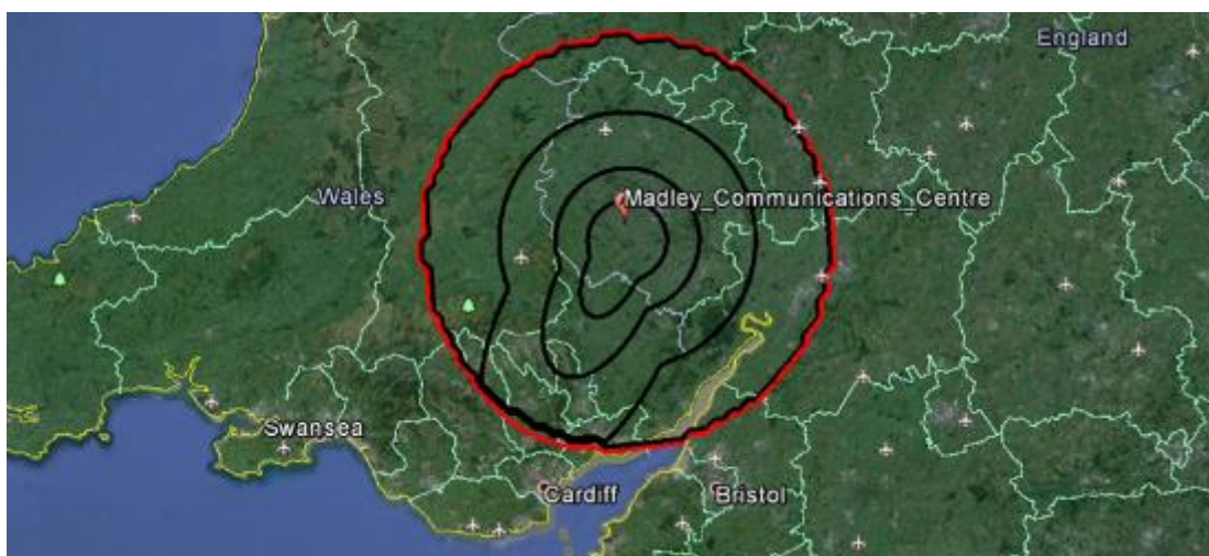
Smooth earth I/N contours derived using Recommendation ITU-R P.452-12
