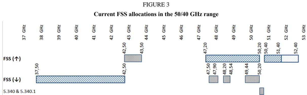
The total bandwidth of primary allocations to unplanned FSS (Earth-to-space) in the bands 40 GHz and 50 GHz in Regions 1, 2 and 3 reaches 5 GHz. In addition, RR No. **5.552** specifies that “Administrations are urged to take all practicable steps to reserve the band 47.2-49.2 GHz for feeder links for the broadcasting-satellite service operating in the band 40.5-42.5 GHz”.
