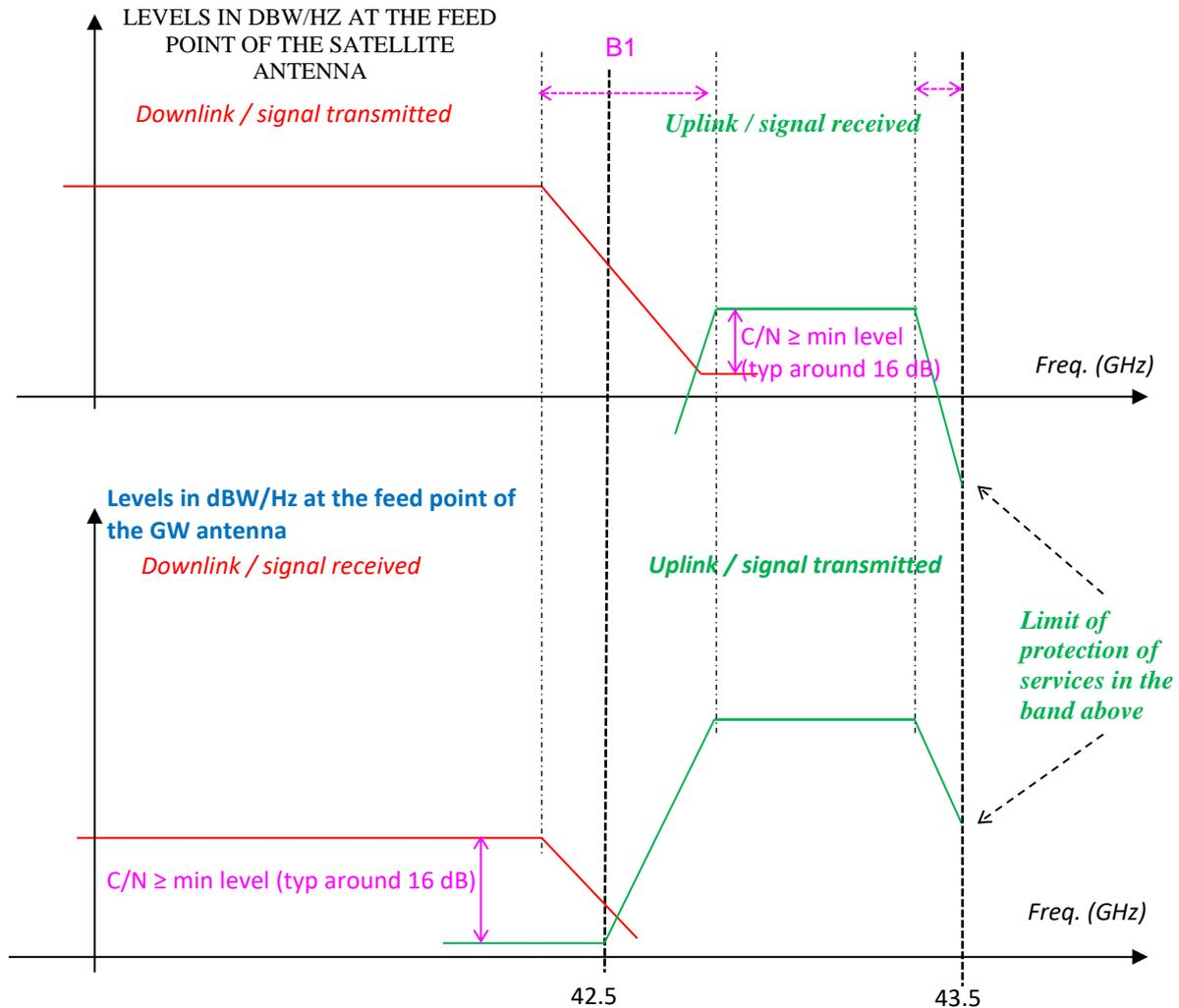
The two uplink allocations to the FSS in the 42.5-43.5 GHz and 47.2-50.2 GHz frequency bands are separated by almost 4 GHz, which leads to the need of an additional frequency conversion, which creates additional intermodulation products, requiring complex filtering systems.
