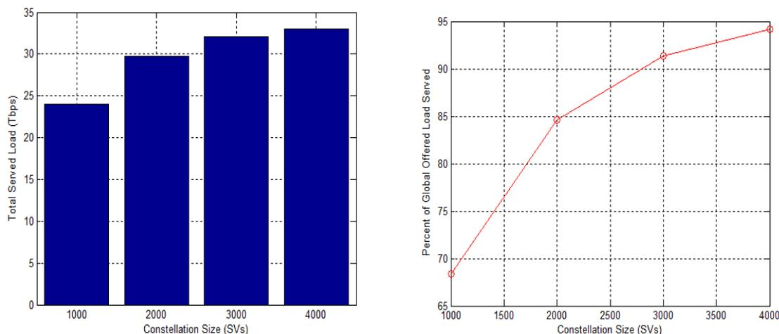
As can be seen by Fig. 8, a non-GSO network operating with a full 5 GHz of spectrum available for both the uplink and downlink could provide global broadband capacity to service unserved and underserved regions of the world. Satellite services can be used to provide this service and to help bridge the broadband digital divide within the next decade.
