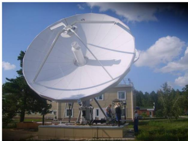
FIGURE 19 7.3 m Antenna system
