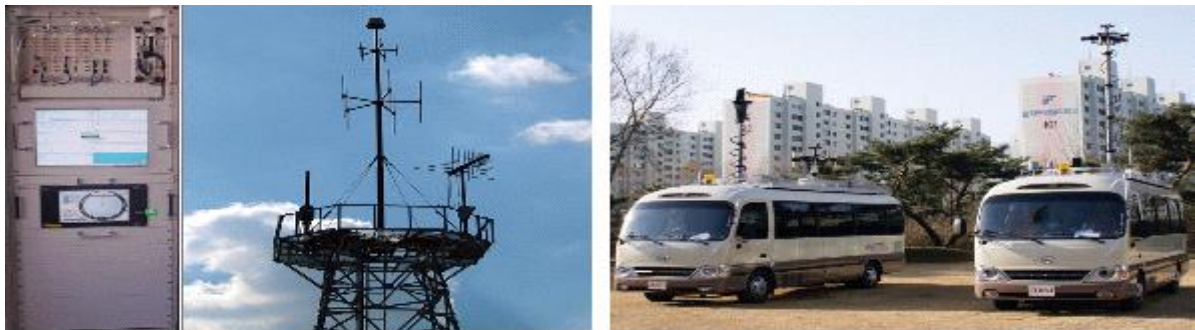
FIGURE 20 Used fixed (left) and mobile (right) monitoring system to measure the spectrum occupancy
