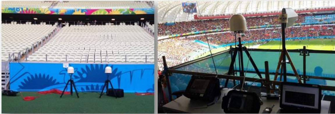
Anatel Spectrum monitoring stations installed at the 2014 World Cup stadiums
