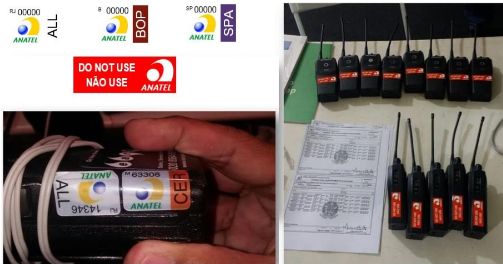
Examples of tags, tagged RF equipment and mobile radios tagged with "Do not use" red tags
