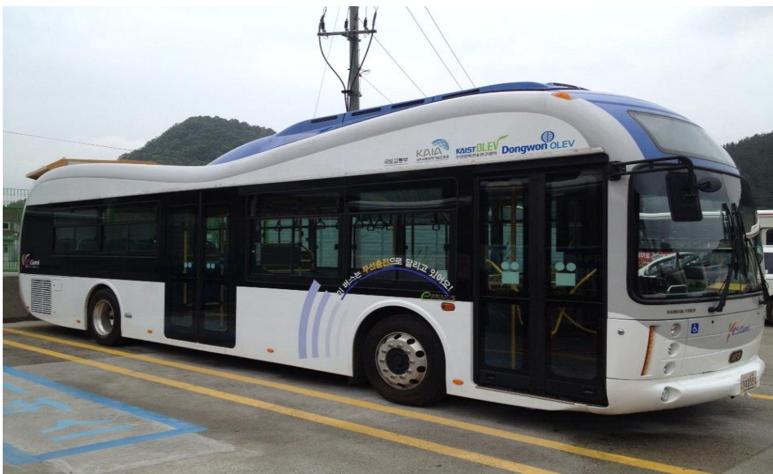
FIGURE 10 Example of an online electric vehicle
