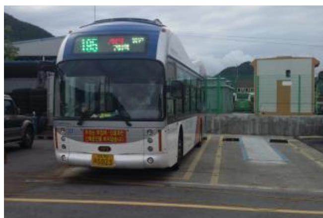
FIGURE A4-5 WPT bus and charging area (right hand side)
