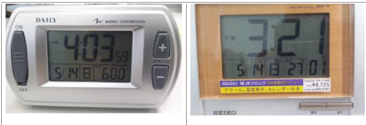
Real clocks used 60 kHz standard time signal
