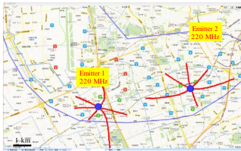
FIGURE A2-10 Co-frequency signals spatial separation (Emitter pairwise distance is 4.1 km)
