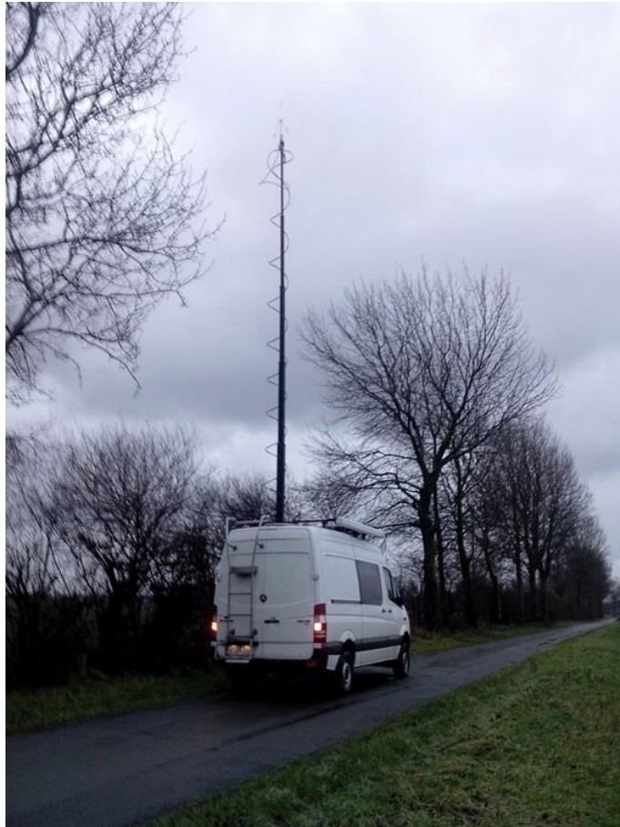
Monitoring vehicle with 10 m mast and transmitting antenna
