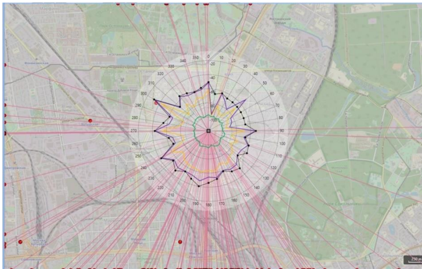
FIGURE 7 Directions to emission sources, based on measurement data (red lines)
