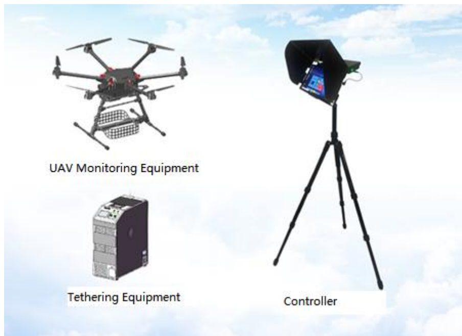
FIGURE 3 Monitoring system structure based by UAV
