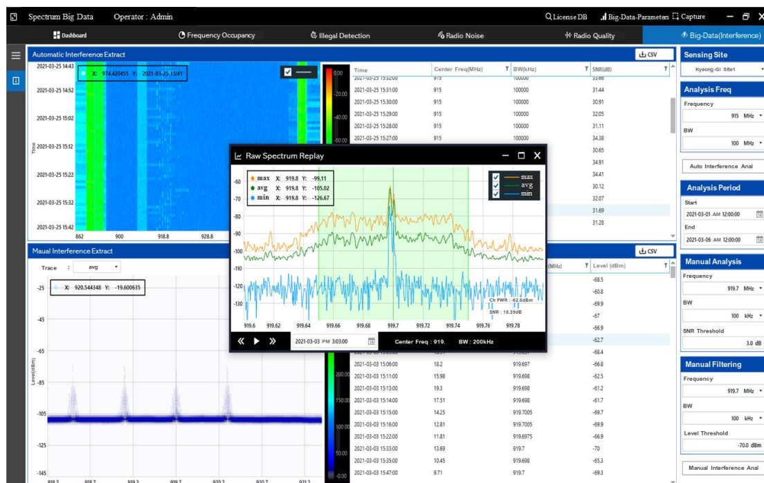
Spectrum monitoring with local processing for illegal transmission and interference detection
