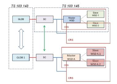
Objective A: CRS including WSD and devices under LSA – TVWS activity and geo-location databases
