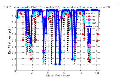
Fig. 12. Average probability of detection at different locations for channel 45. This channel is clearly visible in some locations and not in others. Local sensing fails in reliably detecting this channel while cooperative sensing does.
