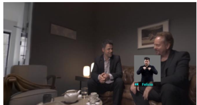
Fig. 5 – Presentation of sign language video, with arrows and speaker's name (and color)
