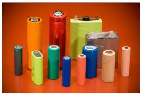
Cylindrical/Prismatic metal case (steel / aluminium). Robust, Easy packaging, Expensive, Jelly roll or stacked electrodes. High energy density, Good heat dissipation,
