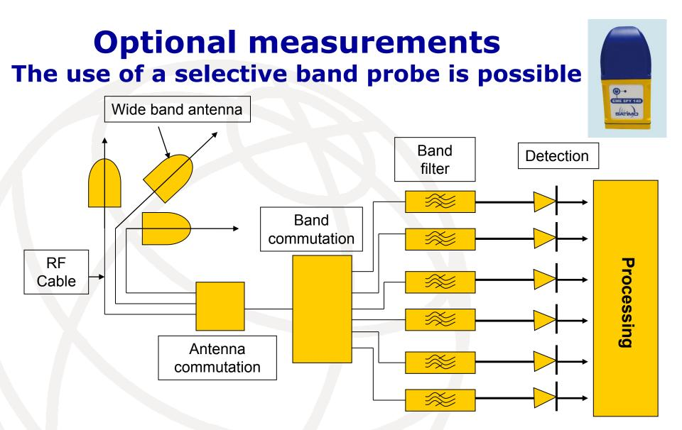
An important criteria for this type of equipment is the selectivity of the filter
