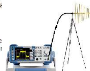
SPECTRUM ANALYSER WITH TRIPOD MOUNTED ANTENNA CONNECTED
