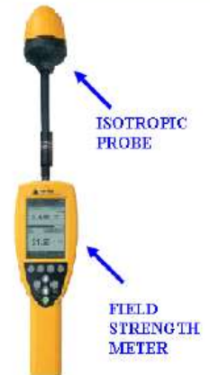
PORTABLE SPECTRUM ANALYSER WITH ANTENNA DIRECTLY CONNECTED
