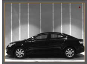
Front speaker used, car well damped, low level outside (1400 - 1800 Hz)
