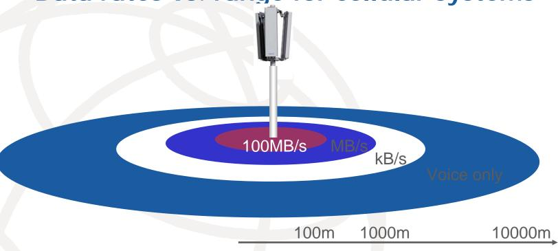
Wide area wireless systems are limited to ~100MB/s Higher data rates are only feasible for local area coverage
