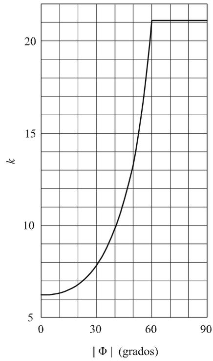
$$k = (2\pi + 4,95 \text{ tg}^2 \Phi) \quad \text{para } |\Phi| \leq 60^\circ$$
